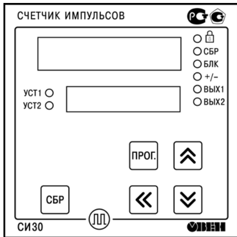
Figure 6.2 – Front panel of the device in housings for wall-mounting H and panel-mounting Щ1
